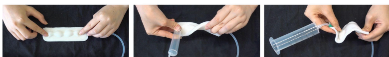
Figure. 1.22. I use deformable silicone bladders to mimic the flexible movement of the vocal cords.
